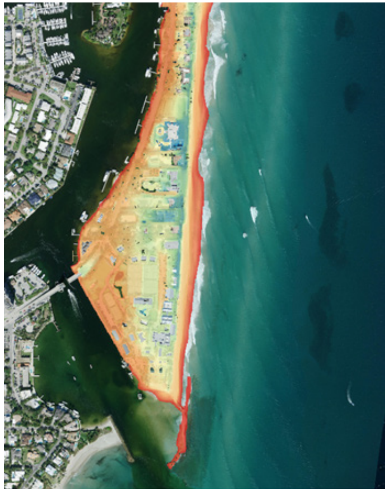
A high-resolution Digital Elevation Model of the southern tip of Hillsboro Beach, near Hillsboro Inlet, capturing detailed terrain elevation, essential for coastal analysis and modeling.
