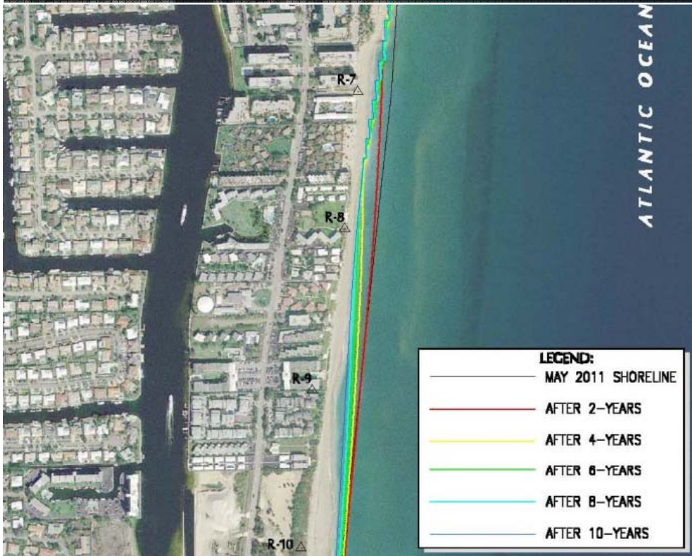
Alternatives 5a and 5b – T-Head Groins into Hillsboro Beach
