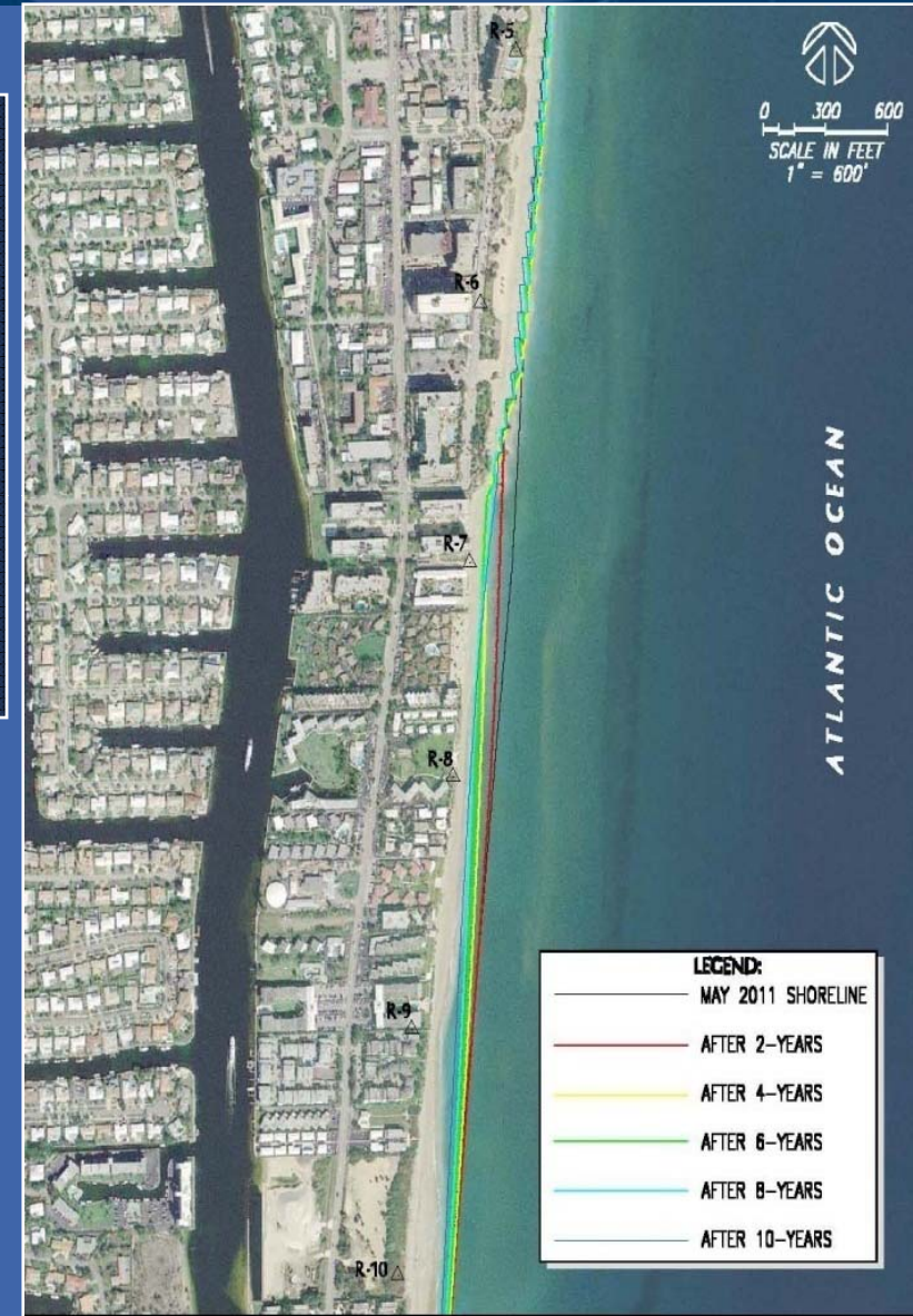
Alternative 3 – Modify Deerfield Groin Field
