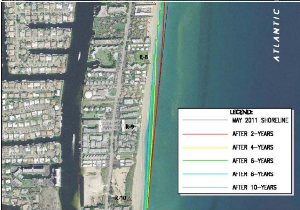
Alternatives 4a & 4b – Groin Field Extension into Hillsboro Beach
