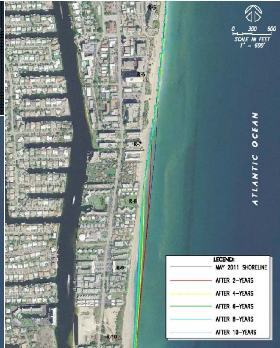
Alternatives 5a and 5b – T-Head Groins into Hillsboro Beach
